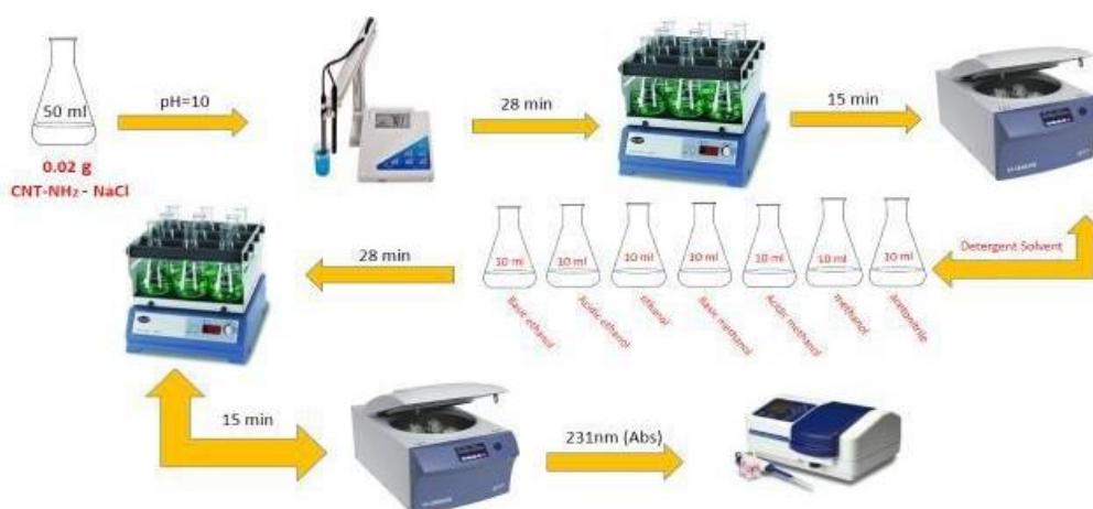
FIGURE 2 Schematic of the quantitative measurement of fluoxetine and determination by UV-Vis spectrometry
