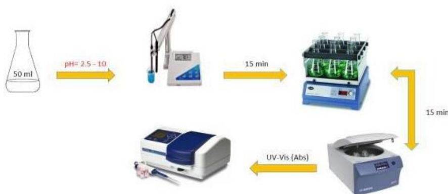
FIGURE 1 The desired drug along with amino-functionalized carbon nanotube absorbent and the buffer range of 2-10 was measured quantitatively by UV-Vis device after centrifugation. Optimizing Wavelength in Fluoxetine Extraction
