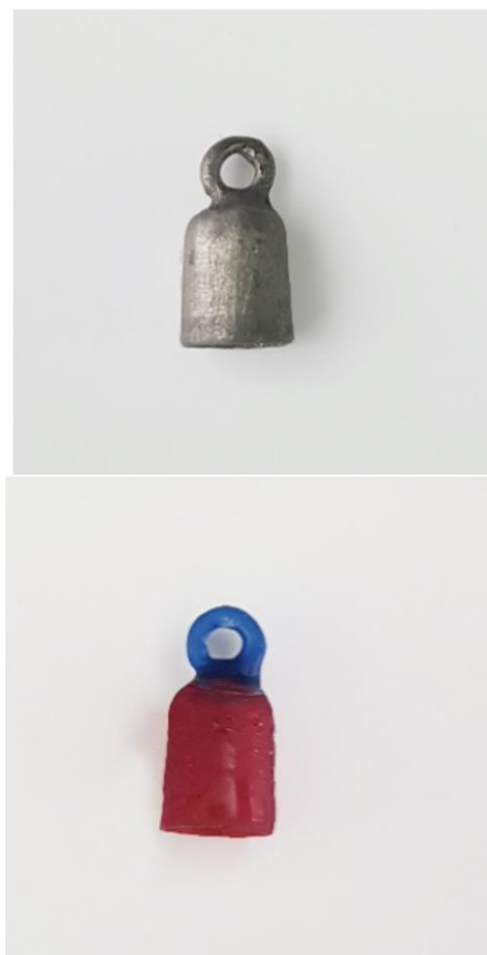
FIGURE 2 Resin template rendered by 3D printer (right) and final casting coping (left)
