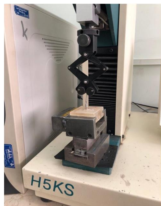
FIGURE 5 Under tension specimens in the universal test machine
