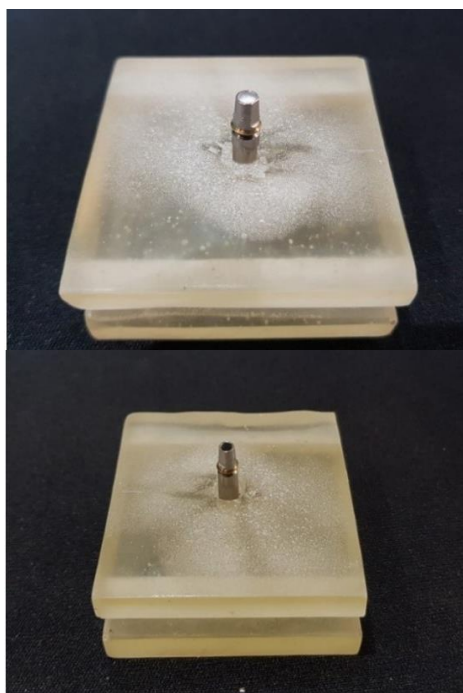
FIGURE 3 Set of abutment and analog mounted in acrylic block (right) and occlusion of the access hole of the abutment screw using temporary filler (left)
