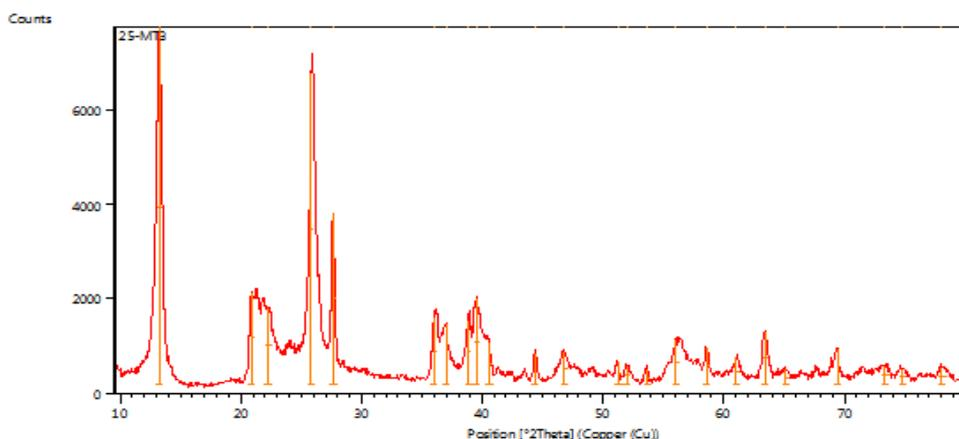
**FIGURE 3** XRD spectrum of kao/Al surface
