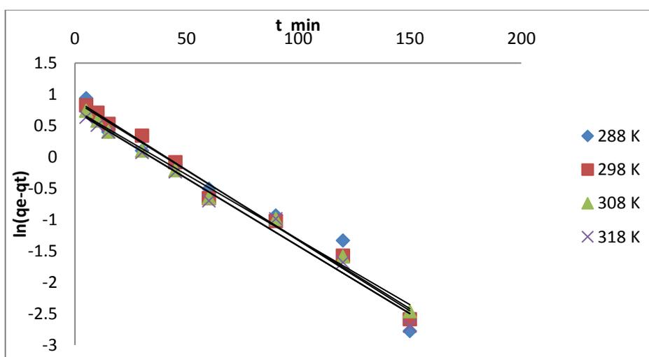
**FIGURE 11** The pseudo-first order kinetic of MG adsorption (50 mg/L) by using kao/Al surface
