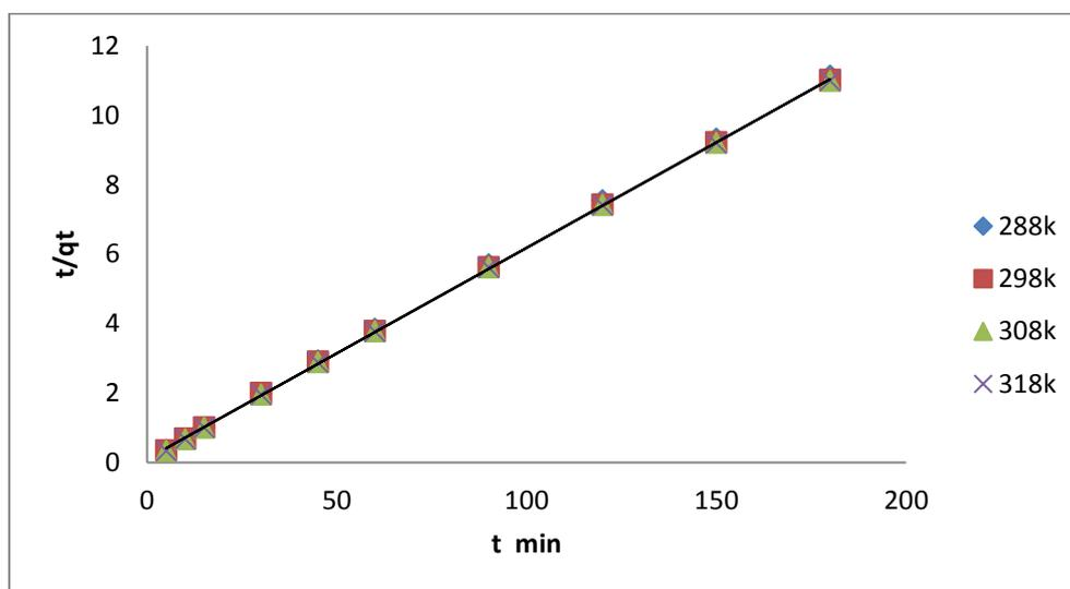
**FIGURE 13** The pseudo-second order kinetic of MG adsorption (50 mg/L) by using kao/Al surface
