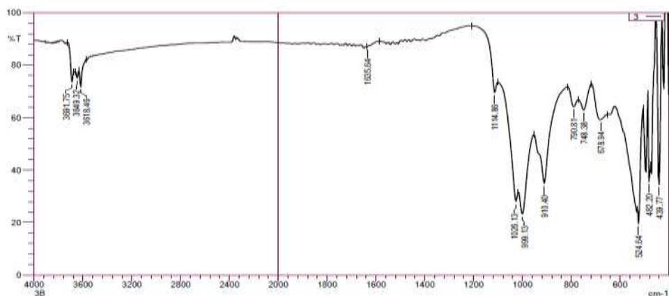
FIGURE 5 FT-IR spectrum of kao/Al surface
