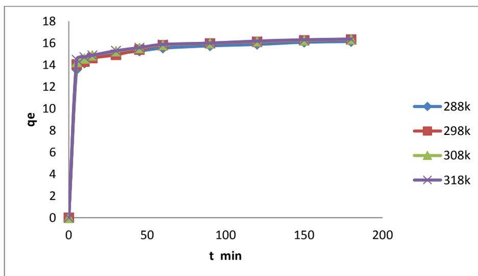
**FIGURE 9** Effect of contact time and temperature on MG dye adsorption (50 mg/L) by kao/Al surface
