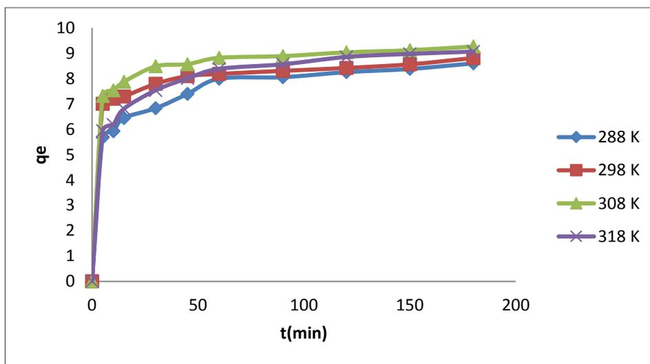
**FIGURE 8** Effect of contact time and temperature on MG dye adsorption (30 mg/L) by kao surface
