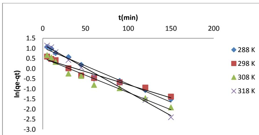
**FIGURE 10** The pseudo-first order kinetic of MG adsorption (30 mg/L) by using kao surface
