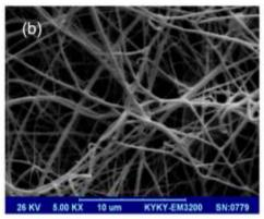
**Figure 4.** SEM images of silk nano-fibres prepared by (a) old chemical method (b) novel physical method
