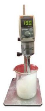
**Figure 1.** Mechanically homogenization with 26000 RPM
