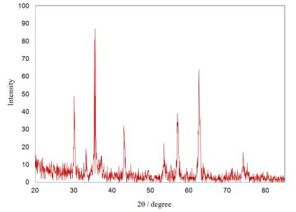
Figure 2. XRD pattern of synthesized CoFe<sub>2</sub>O<sub>4</sub>
